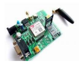
GSM is a worldwide recognised standard for digital cellular communication. A GSM modem is a kind of wireless modem that communicates via a GSM network. GSM SMS techniques play a critical part in this system. GSM SMS messaging is capable of handling a significant volume of transactions in a relatively short period of time.
