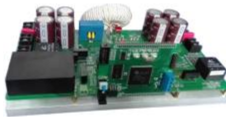
Fig. 9 The experimental prototype of the proposed switched-capacitor bidirectional DC-DC converter.
