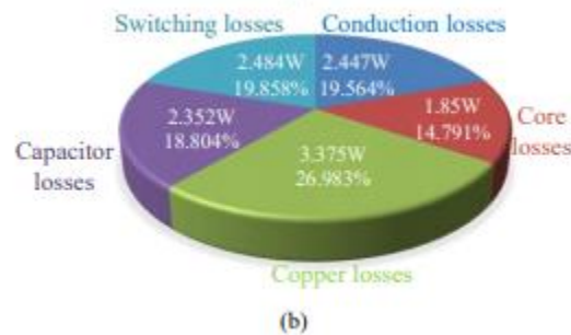
Fig. 22 Calculated power loss distributions for the experiment when U_{low}=40V , U_{high}=300V , and P_n=300W . (a) In step-up mode. (b) In step-down mode.
